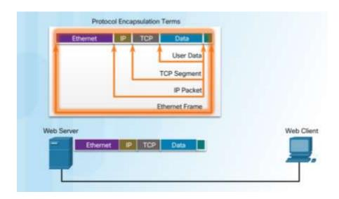
This frame is delivered to the nearest router along the path towards the web client. Each router adds new data link information before forwarding the packet.
